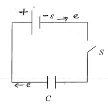
Note: the lines connecting the devices are perfect conductors and so under stationary conditions they must become equipotentials. That is if we close the switch S and wait for a while the Potential difference across C will become  $\varepsilon$ .
