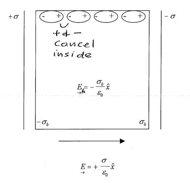
Dipole in E -field experiences torque, which causes each Dipole to line up along E.
