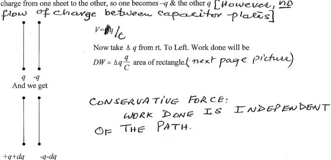
To build up charge from 0 to Q you need area of  $\Delta$  . This work is now  $U_E = \frac{1}{2} \cdot Q(Q/C) = \frac{Q^2}{2C}$
