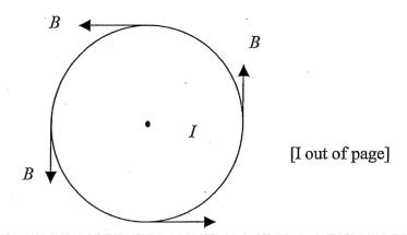
Looking end on (see picture) we have cylindrical symmetry so B can be a function of r only. It turns out that  $B = \frac{\mu_0 I}{2\pi r}$
