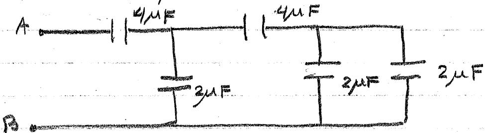
7. Attach a 12V battery across AB. Calculate the charge on each capacitor.
