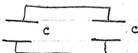
4. Given a capacitor filled with a dielectric,  $C_d = \frac{k\epsilon_0 A}{d}$ . Connect it to a battery and charge it to  $\pm Q$ . How much energy is stored in  $C_d$ ? Disconnect battery. Remove the dielectric. Now how much energy is in  $C_0$ ? Where did the extra energy come from?
