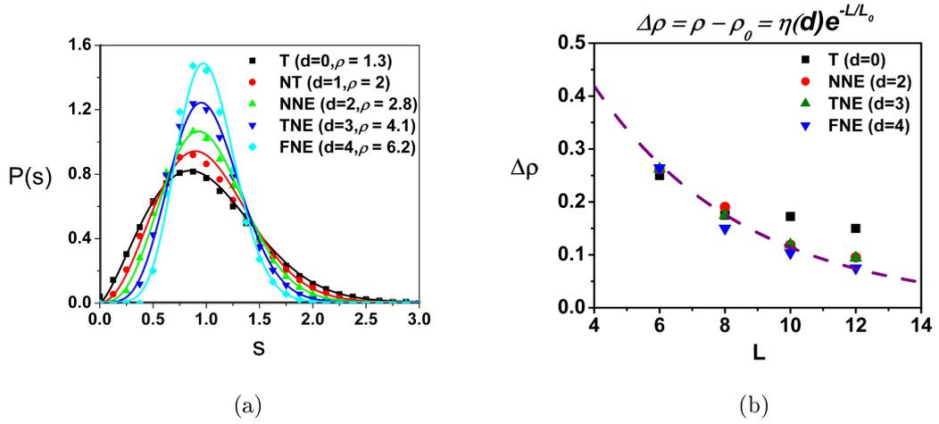
Figure 1: TWDs computed using Monte Carlo simulations: (a) generalized Wigner fits to TWDs of steps with different short-range behavior (b) finite-size effects in interaction strength measurements.
