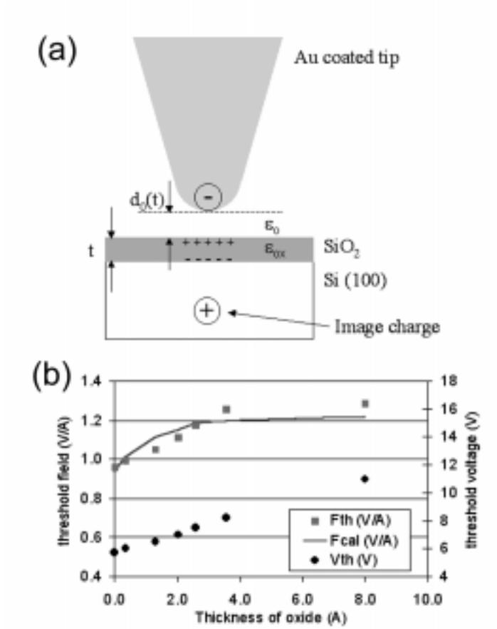
Figure 3 (a) Schematic showing the screening of the attractive force between image charges by oxide. (b) Measured threshold voltage ( $V_{\text{TH}}$ ), corresponding threshold field ( $F_{\text{TH}}$ ), and calculated threshold field ( $F_{\text{CAL}}$ ) versus the oxide thickness.
