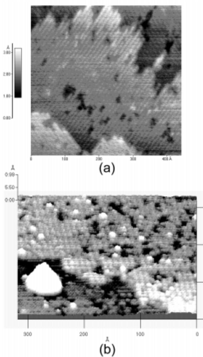
Figure 1(a) STM image of a Si (100) dimer row reconstructed surface taken with a Au coated tip. The density of defect is less than 3 %. (b) Au dot on a partially oxidized silicon surface whose size is 7 nm and height is 10 Å. The tip regenerates and shows an atomic resolution image after making Au dots.
