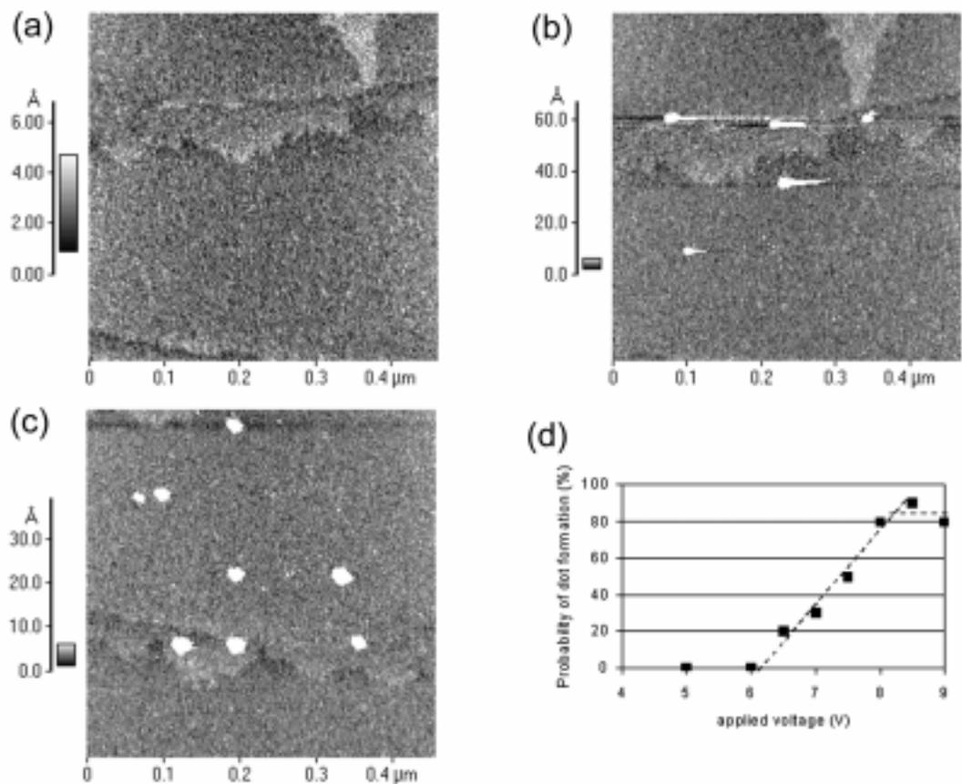
Figure 2. (a)-(c) STM images of oxidized Si (100) after application of multiple voltage pulses between sample and tip. Silicon oxide coverage is 2.2 ML. For these images 10 voltage pulses were applied with heights of -6 V(a), -7.5 V (b), and -9 V (c) to the tip. (d) The probability of dot formations as a function of applied voltage. The threshold voltage is determined to be  $-8.2$  V.
