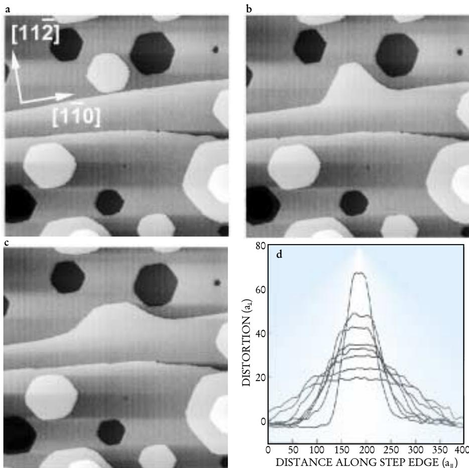
**FIGURE 4. DECAY OF A MONATOMIC ISLAND** on a  $90 \times 90$  nm sample of copper (111) surface at a temperature of 303 K, as viewed with scanning tunneling microscopy. The island suddenly attaches to the step edge forming a bump (a and b) and then decays in time (c) due to edge diffusion, which is shown graphically in (d) with 100-second time steps. (Adapted from M. Giesen, G. S. Icking-Konert, *Surface Science*, volume 412/413, page 645, 1998.)
