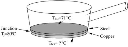
The diagram shows a cross-section of a pan's base. It consists of two layers: a top layer of steel and a bottom layer of copper. The top surface of the steel is labeled  $T_{\text{top}} = 71^\circ\text{C}$ . The interface between the steel and copper is labeled "Junction" with  $T_j = 80^\circ\text{C}$ . The bottom surface of the copper is labeled  $T_{\text{bot}} = ?^\circ\text{C}$ . A handle is shown extending from the right side of the pan.
