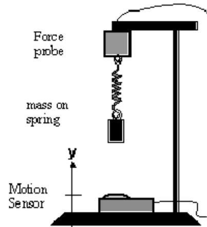
B. Your instructor will lift the mass hanging up, away from the detector, and release it from rest. On these axes, sketch your prediction of the position vs. time as it goes back and forth once.
