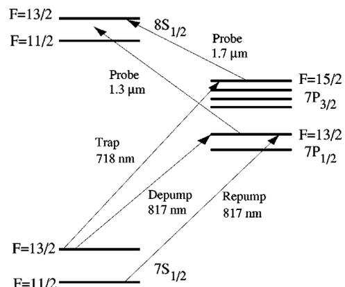
FIG. 1. Diagram of energy levels of  $^{210}\text{Fr}$  relevant for trapping and two-photon excitation.
