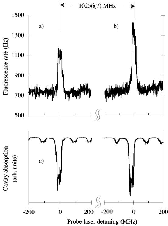
FIG. 4. (a) Fluorescence at 718 nm from excitation to the  $8S_{1/2}$ ,  $F=11/2$  state vs the 1.3- $\mu\text{m}$  laser frequency detuning. The zero of the scan corresponds to  $7494.757 \pm 0.003 \text{ cm}^{-1}$ . (b) Fluorescence from the  $8S_{1/2}$ ,  $F=13/2$  state vs the 1.3- $\mu\text{m}$  laser frequency detuning. (c) Étalon signals with 100-MHz markers.
