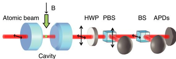
FIG. 2 (color online). Simplified diagram of the apparatus for measuring autocorrelations with an atomic beam in the presence of a magnetic field  $B$ . HWP, half wave plate; PBS, polarizing beam splitter; BS, beam splitter; APD, avalanche photodiode.
