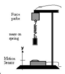
B. Your instructor will lift the mass hanging up, away from the detector, and release it from rest. On these axes, sketch your prediction of the position vs. time as it goes back and forth once.
