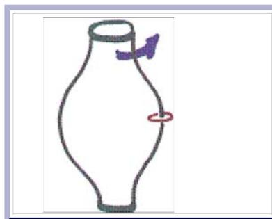
Can a tokamak be optimized? Are there other confinement configurations that might be better from a reactor design viewpoint? The Maryland idea for plasma containment is to spin the plasma. Imagine sliding beads on an electromagnetically spinning, "shaped coat-hanger" magnetic field line. As the beads spin, they gravitate (as it were) to the middle of the shaped field and stay there. Thus, even though the field lines are not closed, the plasma cannot escape. An "open"
