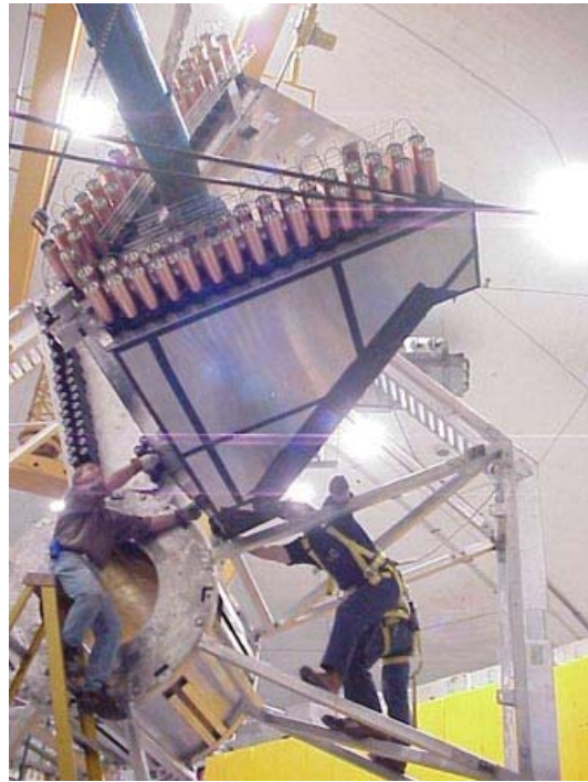
Figure 3b: Two detectors being installed in the support frame (two-octants.jpg).
