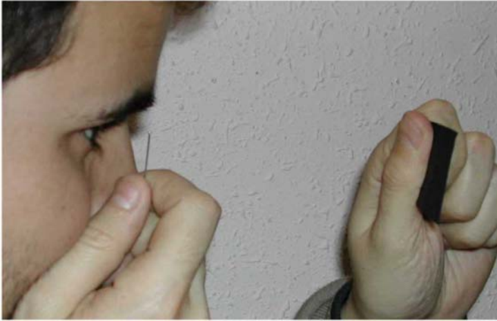
Figure 2. Position of the cardboard and the pin to observe the inverted shadow.
