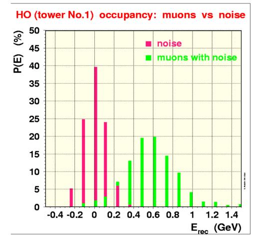
Expect ~ 2 p.e. of noise and ~ 8 p.e. of signal for a single muon at normal incidence.
