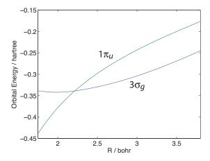
FIG. 15. Variation with distance of the energies of the  $3\sigma_g$  and  $1\pi_u$  orbitals of C<sub>2</sub> determined from complete-active-space (CAS) SCF calculations.
