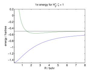
FIG. 1. Electronic energy (blue) and effective nuclear potential (green) for  $H_2^+$  determined from an LCAO-MO wavefunction with  $\zeta = 1$ .
