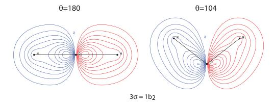
FIG. 21. Contour plot of the  $3\sigma(1b_2)$  orbital of H<sub>2</sub>O in linear (left panel) and bent (right panel) geometry.
