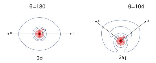
FIG. 20. Contour plot of the  $2\sigma(2a_1)$  orbital of  $H_2O$  in linear (left panel) and bent (right panel) geometry.
