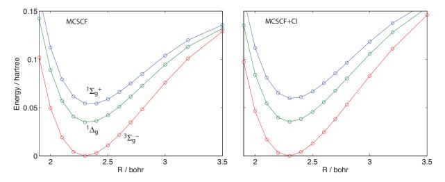
FIG. 12. Electronic potential curves for  $O_2$  determined with complete-active-space (CAS) SCF calculations (left panel) and with CASSCF+CI calculations (right panel).
