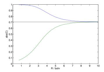
FIG. 6. Calculated coefficients  $C_g$  (blue) and  $C_u$  (green) in the two-configuration MCSCF approximation to the H<sub>2</sub> electronic wavefunction. The absolute values of the coefficients are shown. The sign of  $C_u$  is opposite to that of the sign of  $C_g$ .
