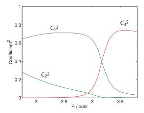
FIG. 14. Variation with distance of the square of the larger coefficients in the expansion of the wavefunction [see Eq. (25)] for the  $^{1}\Sigma_{g}^{+}$  state of C<sub>2</sub> determined with complete-active-space (CAS) SCF calculations.
