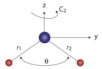
FIG. 18. Geometry of an HMH hydride. The x axis is perpendicular to the plane of the figure. The symmetry elements are  $C_2$ , a two-fold rotation around the z axis;  $\sigma_v$ , a reflection in the xz-plane (the plane that bisects the molecule; and  $\sigma'_v$ , a reflection in the yz-plane (the plane containing the molecule).
