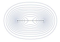
FIG. 3. Contour plot of the lowest  $1\sigma_g$  orbital of H<sub>2</sub>, for an H–H internuclear separation of 1.4 bohr
