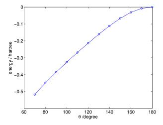
FIG. 25. The sum of the orbital energies of the  $3a_1$  and  $1b_2$  orbitals of  $H_2O$  (see the right panel of Fig. 19), multiplied by two, as a function of the HOH angle.
