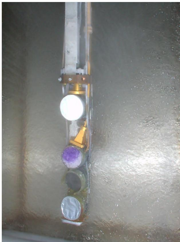
Figure 5.9: Target ladder carrying target cells. The targets are (from top to bottom): top  $^{15}\text{ND}_3$  (the purple spot is due to the radiation damage), 10 mm hole, 8 mm hole (partially obscured by the microwave horn of the bottom  $^{15}\text{ND}_3$  cell), bottom  $^{15}\text{ND}_3$ , carbon and empty.
