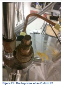
Figure 29: The top view of an Oxford 8T magnet showing the magnet current leads and pressure equalization tubes (copper).
