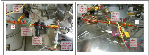
Figure 13: (a) The purified gas enters the liquefier input assembly on the 150L dewar. The point marked "12" corresponds to the same point on the liquefier manifold diagram in Figure 10. (b) The 150L dewar liquefier exhaust assembly sends gas to point number "13" on the liquefier manifold diagram in Figure 10. The coil allows for thermal expansion and contractions without stressing rigidly attached joints.
