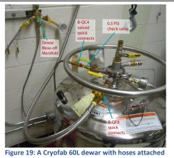
Figure 19: A Cryotab 60L dewar with hoses attached to the vent and exhaust ports. The 0.5 PSIG relief valve has been replaced with a 2 PSIG check valve.
