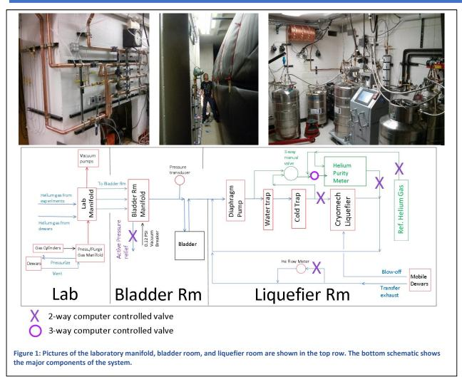
A full laboratory helium recovery system has been implemented to mitigate the burgeoning cost of liquid helium. Laboratory applications require cooling samples, superconducting magnets, and optical detectors down to temperatures below 2K, which requires liquid helium.
