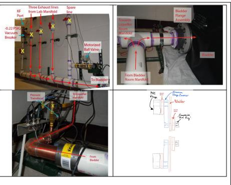
Figure 21: Pictures show (a) the Bladder room manifold, (b) the Bladder room manifold interface with the bladder, and (c) the Bladder send line to the Liquefier manifold showing the pressure transducer and connectors. (d) A sketch of the custom-designed bladder flange assembly.
