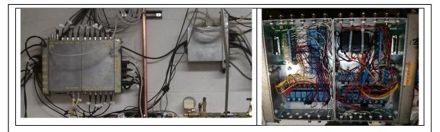
Figure 30: (Left) Electronics box #2 is the larger box on the left, and electronics box #1 is the smaller box on the right. (Right) Inside electronics box #2 are two DB-25 screw-terminal connector blocks, three 8-channel relay boards, three 4-channel k-type thermocouple amplifiers with virtual cold junction offset correction, three dc power supplies, and two 6-outlet power strips.
