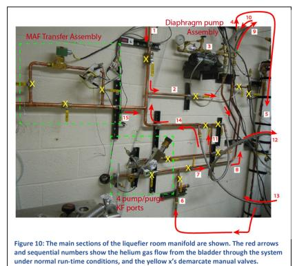
pressurizes the upstream components to around 5 PSIG. From the pump assembly, the helium flows through a check valve (4). The check valve maintains the upstream components above atmospheric pressure when the pump is off. The helium then flows through a flexible corrugated stainless-steel hose, and to the top of the water trap.
