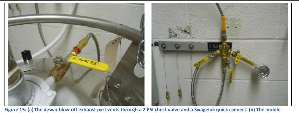
Figure 15: (a) The dewar blow-off exhaust port vents through a 2 PSI check valve and a Swagelok quick connect. (b) The mobile dewars vent into the dewar helium blow-off capture manifold. This manifold attaches directly to the liquefier 150L dewar reservoir.
