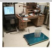
Figure 20: A 440-lb capacity platform scale with an LCD display and RS-232 port connects to the helium recovery system computer.
