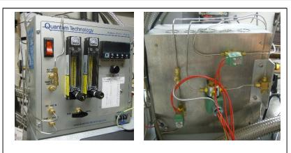
Figure 3: Three computer controlled solenoid valves are mounted to the back of the helium purity meter to automate readings.
