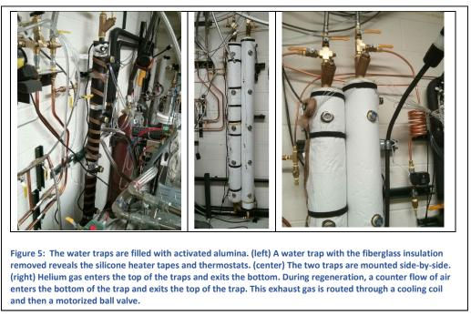
The helium from the bladder and diaphragm pump is routed through water traps. The traps are filled with beads of activated alumina. Blue indicating activated alumina is packed into windows along the length of the trap. The trap is conveniently regenerated *in situ* by heating and flowing air across the bed.
