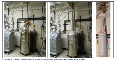
Figure 6: The cold trap is removed from the liquid nitrogen bath.
