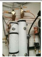
Figure 11: The top of each water trap has an input isolation valve (top) and a manual exhaust port valve (side).
