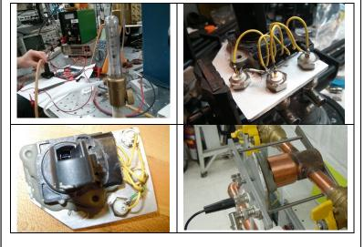
Figure 16: Modified automotive Mass-air-flow sensors are used as adjustable helium flow sensors and the Laboratory and Liquefier manifolds
