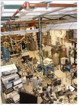
Figure 28: Laboratory laser-area pipeline with five KF-40 ports that interfaces with flexible hose that hang from the ceiling and attach to experiments.
