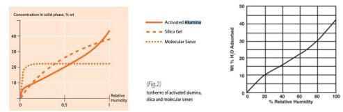
Activated alumina was chosen over silica gel, activated charcoal, and zeolites/molecular sieves. At low relative humidity, the case for recovered helium, zeolites are the most efficacious for adsorbing water. However, the extremely high bake temperature (>300C) makes regeneration difficult. Activated alumina is better than silica gel at low relative humidity and regenerate at relatively low temperatures, >150C. Also, the water capacity of activated alumina is high.
