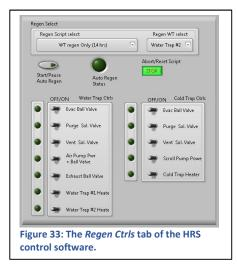
Regeneration of the water traps and cold trap was described in section *Liquefier room* subsections *Water traps* and *Cold trap*. Both traps during the regeneration process are heated, purged with industrial grade helium, vented, and evacuated. The water traps are flushed with a counter flow of ambient air while hot.
