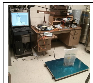
Figure 18: A 440-lb capacity platform scale with an LCD display and RS-232 port connected to the liquefier computer.
