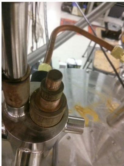
Figure 27: Top of 8T magnet showing the magnet current leads and pressure equalization tube (copper).
