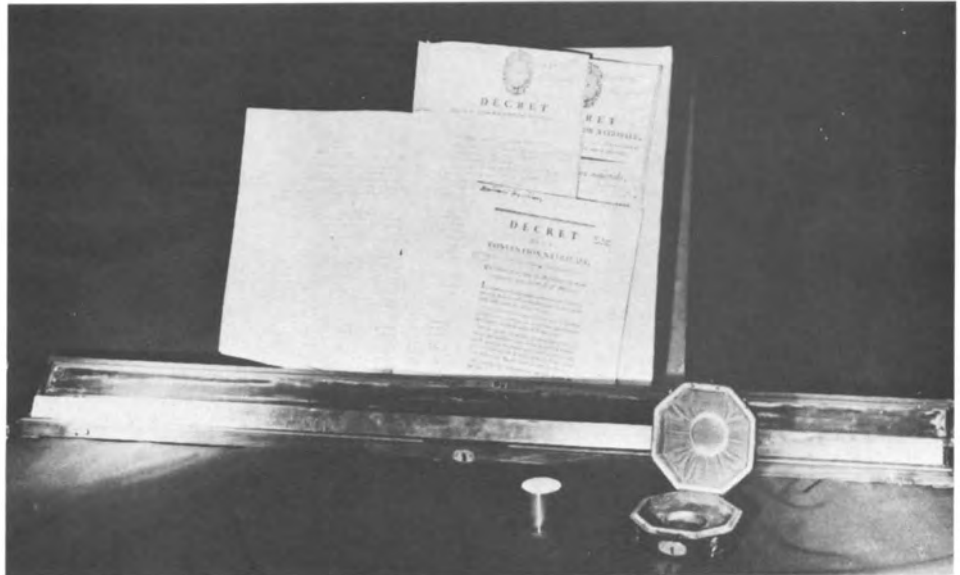
Fig. 5. Mètre et Kilogramme des Archives of 1799, a platinum bar and cylinder deposited in the Archives de la République . These standards served as the legal representations of the metric units. In the background are the decrees of 1793 and 1795 which established the metric system in France. (Photo Archives Nationales, Paris.)
