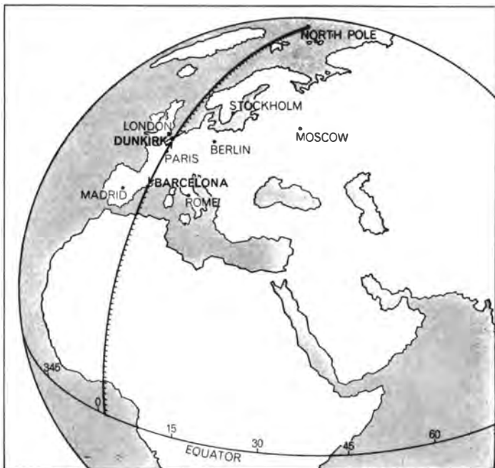
Fig. 1. Portion of quadrant of the earth surveyed between Dunkirk and Barcelona. From measurements of star positions the difference in latitude was determined, permitting extrapolation of the actual distance measured to the entire quadrant. The meter was defined as the length of one ten-millionth of the earth's quadrant. (From "Standards of Measurement" by Allen V. Astin. Copyright © June, 1968 by Scientific American, Inc. All rights reserved.)
