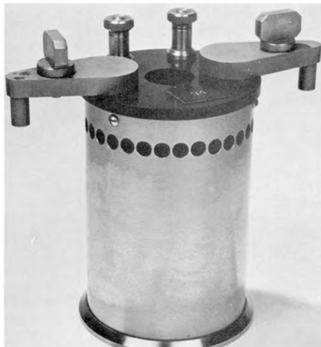
Fig. 17. Standard 1- \Omega resistor. The outer terminals are for current and the inner terminals are for potential difference. With this arrangement the effect of the resistance of the leads can be eliminated. This resistor is of the double-walled or Thomas-type. A bifilar coil of manganin wire is wound on a tubular form hermetically sealed in dry air within the outer container. The series of holes near the top are above the sealed space and facilitate cooling by an oil bath. Since 1939 a bank of 10 similar resistors has been used to maintain the ohm at the National Bureau of Standards. Resistance was calibrated by comparison with the reactance of a known frequency of a large inductor whose self-inductance could be calculated from its dimensions and the assigned permeability of free space \mu_0 . However, resistance standards are now calibrated by comparison with the reactance of a calculable capacitor, a method made feasible in 1956 by the Thompson-Lampard theorem of electrostatics. Only a single measurement of length is required. (The permittivity of free space \epsilon_0 must also be known but this is given by \epsilon_0 = 1/\mu_0 c^2 .) According to a determination made in 1974 the NBS ohm was equivalent to 0.999 999 18 absolute ohm with an uncertainty of \pm 0.06 part per million. (National Bureau of Standards photo.)
