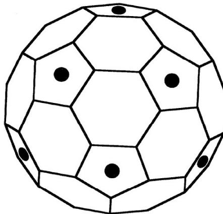
Figure 1: Truncated icosahedral arrangement of transducers
