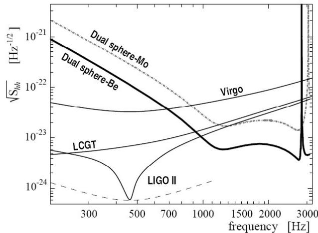
Figure 3: Plot of estimated sensitivity of dual sphere detector
