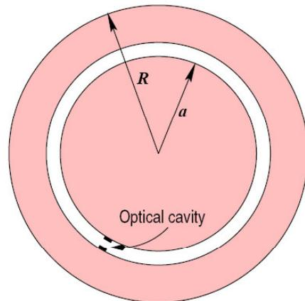
Figure 2: Dual spherical detector
