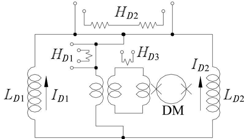
(a) DM sensing circuit
