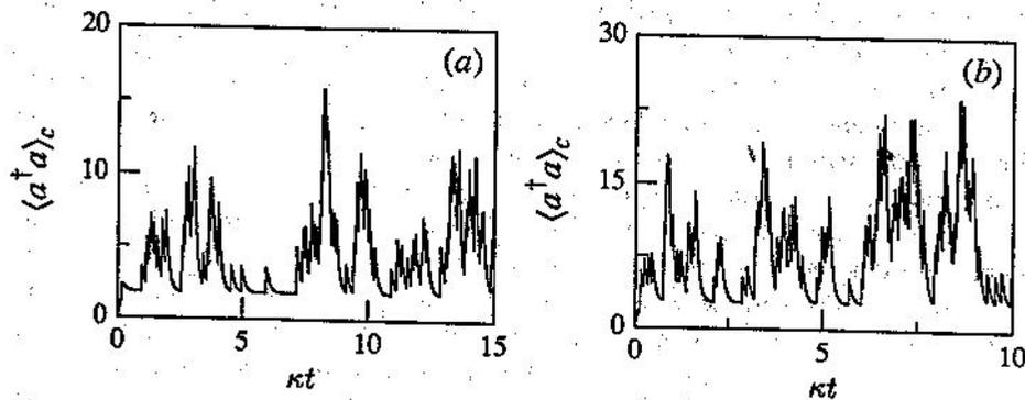
Fig. 8.7. Sample quantum trajectories showing the conditioned mean photon number for a cavity driven by thermal light. (a) The thermal light turns on at  $t = 0$  and injects a photon flux  $2\kappa\bar{n} = 10\kappa$  ( $\bar{n} = 5$ ). The Fock state basis is truncated at 50 photons. (b) The thermal light turns on at  $t = 0$  and injects a photon flux  $2\kappa\bar{n} = 20\kappa$  ( $\bar{n} = 10$ ). The Fock state basis is truncated at 80 photons.
