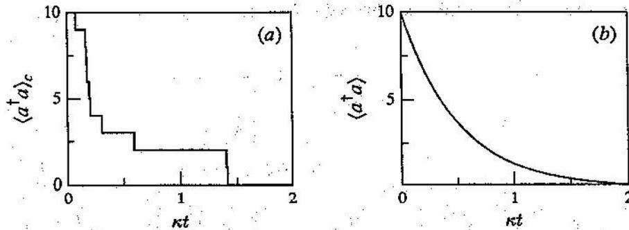
Fig. 8.2. (a) Sample quantum trajectory showing the conditioned mean photon number for a damped cavity mode prepared in the Fock state  $|10\rangle$ . (b) Average of the conditioned mean photon number for 10,000 trajectories.
