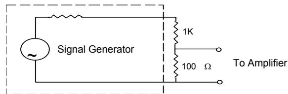
8. The measurement of the a.c. gain of a circuit implies that the output is a linear function of the input. Normally this is the case if the circuit under test is not overloaded to the point where the output signal is distorted. Gain measurements are best made with an oscilloscope where the input and output waveforms can be observed simultaneously.
