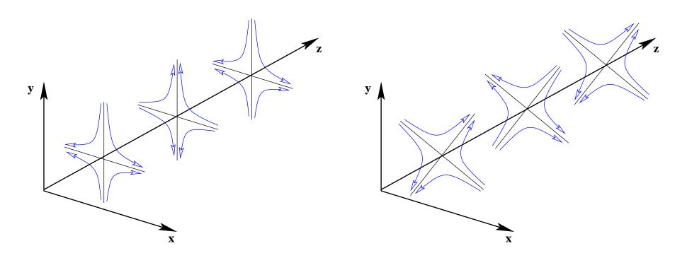
Force pattern of GWs are invariant under  $180^{\rm o}$  degree, by contrast force patterns of EM waves are invariant under  $360^{\rm o}$  degree
