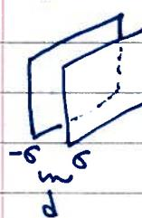
$$\begin{aligned} \text{outside: } \vec{E} &= 0 \\ \text{inside: } \vec{E} &= -4\pi\sigma \hat{z} \end{aligned}$$
