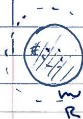
$$\begin{aligned} \text{outside: } 4\pi r^2 E &= 4\pi Q \Rightarrow \vec{E} = \frac{Q}{r^2} \hat{r} \\ \text{inside: } 4\pi r^2 E &= 4\pi Q \frac{r^2}{R^3} \Rightarrow \vec{E} = \frac{Qr}{R^3} \hat{r} \end{aligned}$$
