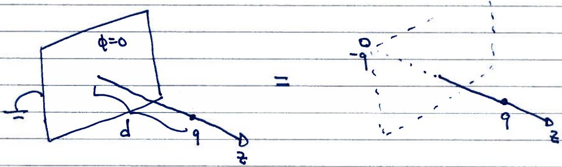
$$\phi(x, y, z) = \frac{q}{\sqrt{x^2 + y^2 + (z-d)^2}} - \frac{q}{\sqrt{x^2 + y^2 + (z+d)^2}}$$
