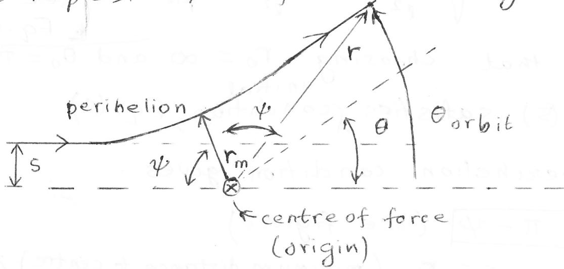
At perihelion, angle between position vector and initial direction of particle is  $\psi$  so that
