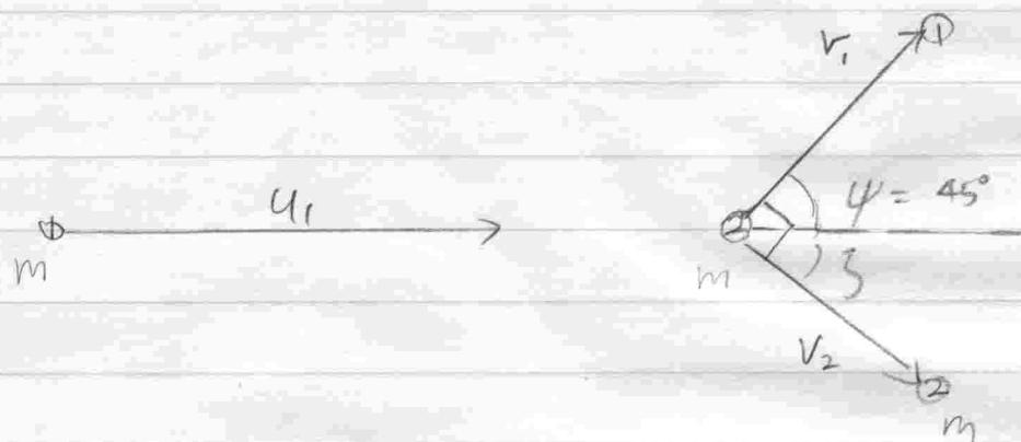
For elastic collisions btwn two same masses, the two emerge with an angle  $90^\circ$  btwn them, so  $\theta = 45^\circ$ .
