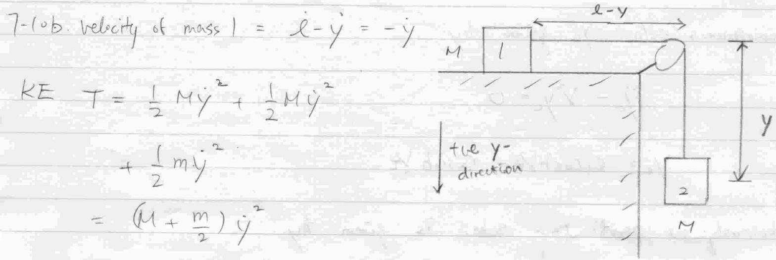
$$\text{KE } T = \frac{1}{2} M \dot{y}^2 + \frac{1}{2} M \dot{y}^2 + \frac{1}{2} m \dot{y}^2 = (M + \frac{m}{2}) \dot{y}^2$$
