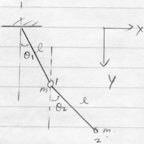
$$\text{KE} \quad T = \frac{1}{2}m(\dot{x}_1^2 + \dot{y}_1^2) + \frac{1}{2}m(\dot{x}_2^2 + \dot{y}_2^2)$$
