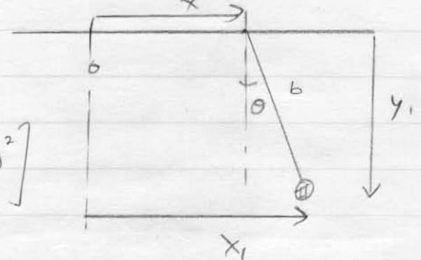
$$\text{KE} \quad T = \frac{1}{2}m[(\dot{x} + b\dot{\theta}\cos\theta)^2 + (b\dot{\theta}\sin\theta)^2] \\ = \frac{1}{2}m[\dot{x}^2 + b^2\dot{\theta}^2 + 2b\dot{x}\dot{\theta}\cos\theta]$$
