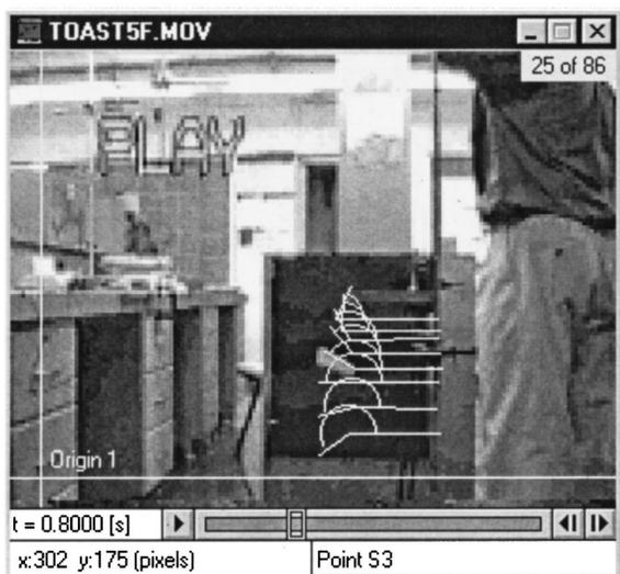
Fig. 5. Experimental setup for measuring the free fall angular velocity as a function of overhang.
