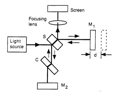
Figure 1: Schematic illustration of a Michelson interferometer.
