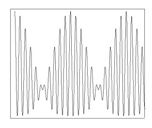
Figure 2: Beat signal from two input frequencies into a Michelson interferometer
