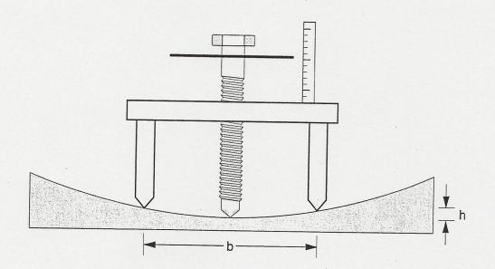
Figure 4: Schematic illustration of how to use a spherometer to measure the radius of curvature of a lens. Note, h measures the difference in the lengths of the center screw and the three feet and b is the length of the side of the triangle formed by the feet. DO NOT USES THE SPHEROMETER ON THE MIRROR!
