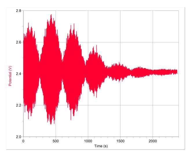
The period of the envelope oscillation was taken to be the average of the distances between peaks for the first 4 peaks. This was found to be 343 seconds which gives a frequency of  $v_{envelope} = 2.915$  mHz. The error in the determination of each peak was 6 seconds. The propagation of this error to the error in  $v_{envelope}$  is direct since  $v_{envelope}$  is an average of the values with this error. The error in  $v_{envelope}$  is 0.167 Hz (1/[6 seconds]).
