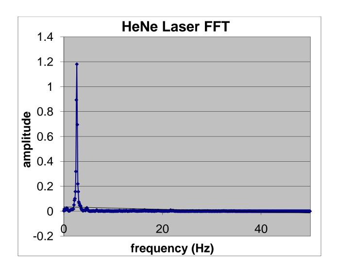
This frequency of fringes (2.64+-0.22 Hz) can be used to find the speed of M1. This is shown below where *speed* is the speed of M1, v is the frequency of fringes, and  $\lambda$  is the wavelength of the HeNe laser light. The speed of M1 is found to be **841 nm/s**.
