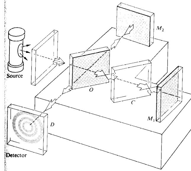
Start with the laser at a fixed height, the beam aligner at a fixed height, the front of the MI at a fixed height and level. (If the heights are messed up, have Tommy reset them.) Then adjust the mirror on the beam aligner to retroreflect. Use the two knobs on the back of the mirror, and adjust the beam height using the knob on the side of the unit. You must both retroreflect the beam and center the beam on the moveable mirror in the MI.
