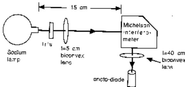
Note that the Na lamp has a limited longitudinal coherence length. Therefore, interference patterns are most easily seen when the two arms of the interferometer are of nearly equal length.
