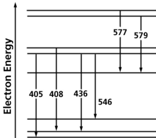
The measured lines of Mercury in the nominal [visible region](#) are:
