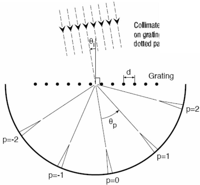
$$p\lambda = d(\sin \theta_p + \sin \theta_i), \quad p = \pm 1, \pm 2, \pm 3, \dots$$
