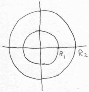
$$\Phi(R_1, \theta) = V_1 (\sin^2 \theta - \frac{1}{2}) = -\frac{V_1}{4} (e^{i2\theta} + e^{-i2\theta})$$
