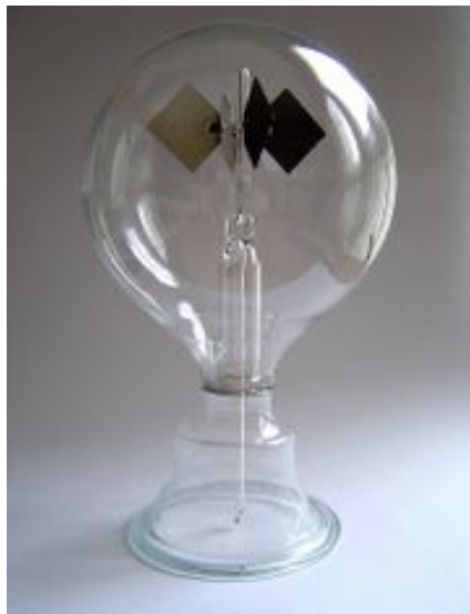
Figure 1: A radiometer or light mill.
