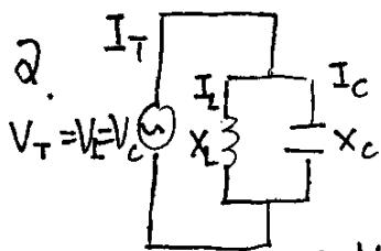
In the pure LC parallel-tuned circuit (that is, one in which there is no resistance), the coil and the capacitor are placed in parallel and the applied voltage  $V_T$  appears across these circuit components. In this parallel-tuned circuit, as in the series-tuned circuit, resonance occurs when the inductive reactance is equal to the capacitive reactance.
