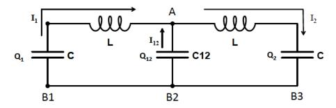
This circuit is the electrical analog of the coupled mechanical oscillators that we studied earlier in the semester (see Homework #5).
