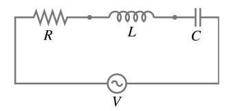
By considering the phasor diagram for the voltages in this circuit, we found the following expression for the circuit impedance:
