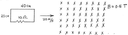
a.) (10 pts.) Calculate the time it takes the loop to enter the field region completely. Then plot the flux that passes through the square loop versus time, t, with t=0 being the time the loop enters the magnetic field. Show on your plot the maximum value of the flux and the time when the loop is inside.
