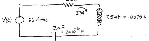
a.) (10 points) Apply Kirchoff's rule to this circuit to obtain an equation that relates the current I(t) to the driving voltage V(t).
