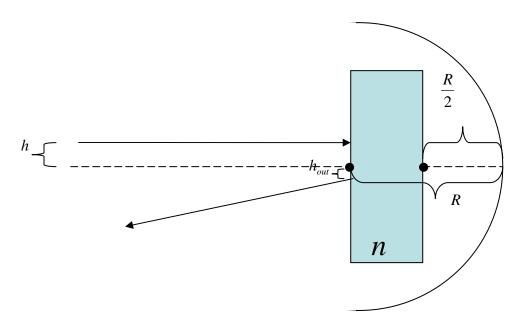
Suppose a ray of light parallel to the symmetry axis and located a distance h above comes in from the left. (You may assume that h is much smaller than R.)The ray passes through the slab reflects from the mirror and passes through the slab a second time. It will ultimately leave the slab some distance  $h_{out}$  below the axis at some angle  $\theta$ . The purpose of the problem is find  $h_{out}$  and  $\theta$ .
