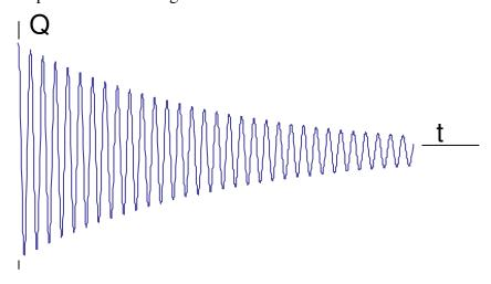
Explain how the qualitative features of this graph such as the distance between neighboring maxima and the rate at which the maxima drop off with t are related to the parameters R L & C..
