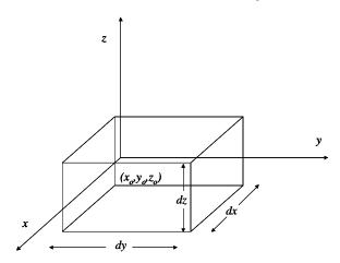
$$-\int F_{x}\left(x_{o},y,z\right)dydz + \int F_{x}\left(x_{o}+dx,y,z\right)dydz$$
