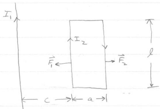
my numbers:  $I_1 = 8 \text{ A}$ ,  $I_2 = 10 \text{ A}$ ,  $l = 0.7 \text{ m}$ ,  $c = 0.1 \text{ m}$ ,  $a = 0.15 \text{ m} \Rightarrow F = 6.72 \times 10^{-5} \text{ N}$
