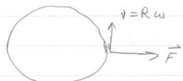
$$\begin{aligned} q\mathcal{E} &= \int_0^R d\vec{r} \cdot \vec{F} \\ \vec{F} &= qB\omega \vec{r} \end{aligned} \quad \left\{ \begin{array}{l} \mathcal{E} = \frac{1}{2}BR^2\omega \end{array} \right.$$
