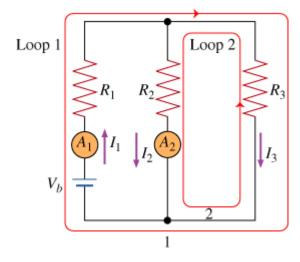
for that current will be negative. The direction of any loop is even less imporant: The equation obtained from a counterclockwise loop is the same as that from a clockwise loop except for a negative sign in front of every term (i.e., an inconsequential change in overall sign of the equation because it equals zero).
