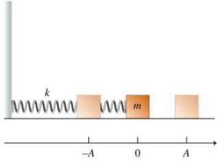
figure . The spring can be either stretched or compressed. The block slides on a frictionless horizontal surface, as
