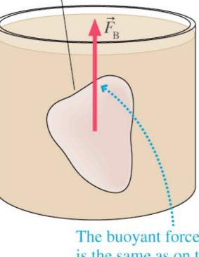
The buoyant force on the object is the same as on the parcel of fluid because the *surrounding* fluid has not changed. The net force of the fluid on the cylinder is the buoyant force  $\vec{F}_{\rm B}$ .
