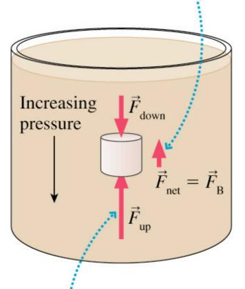
$F_{up} > F_{down}$  because the pressure is greater at the bottom. Hence the fluid exerts a net upward force.
