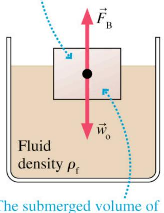
The submerged volume of the object is equal to the volume  $V_f$  of displaced fluid.
