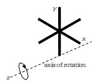
The parallel axis theorem can be used for calculating the contributions of all three rods to the total I.
