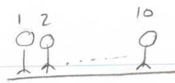
Assume each person weighs  $\approx 50\text{ N}$  (that's  $\approx 110\text{ lbs}$ ) so total weight  $Mg = (10 \times 50\text{ N}) = 500\text{ N}$ . weight of elevator  $\approx (500\text{ kg})(10\text{ m/s}^2) = 5000\text{ N}$
