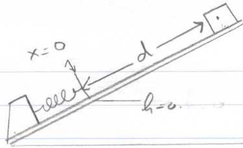
$t_1 \rightarrow t_2$ : Now the block starts compressing the Spring. The gravitational P.E decreases further and so does its K.E. The block comes to rest at  $X$  (momentarily.)
