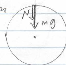
b1. cannot have a tangential acceleration at the top since both the normal force and  $F_g$  point in the radial direction at the top. There is no force in the tangential direction (assuming no friction.)
