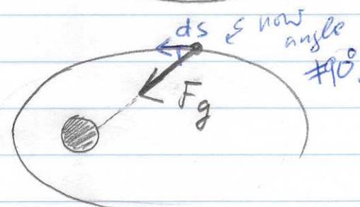
now the work done is not zero. since the satellite moved closer to the earth, (i) the work done by gravity is positive and therefore (ii)  $W_g = \Delta K.E > 0 \Rightarrow K.E_f > K.E_i$  so  $v_B > v_A$ .
