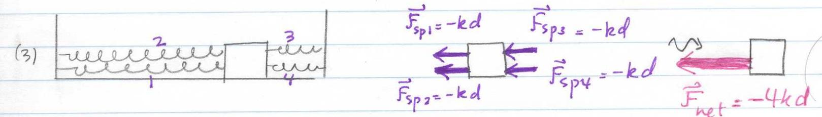
$\Rightarrow |\vec{F}_{net}^{(3)}| > |\vec{F}_{net}^{(2)}| > |\vec{F}_{net}^{(1)}|$ . Note that if the block were displaced to the left, the force due to each spring would be in the opposite direction but its magnitude would still be the same. So the ranking above would be the same.
