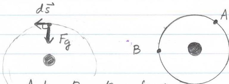
point along its path from A to B, the force on the satellite is perpendicular to its displacement since the displacement at each point is tangential to the circle. So the work done by the force of gravity on the satellite as it moves from point A to B is **ZERO**.
